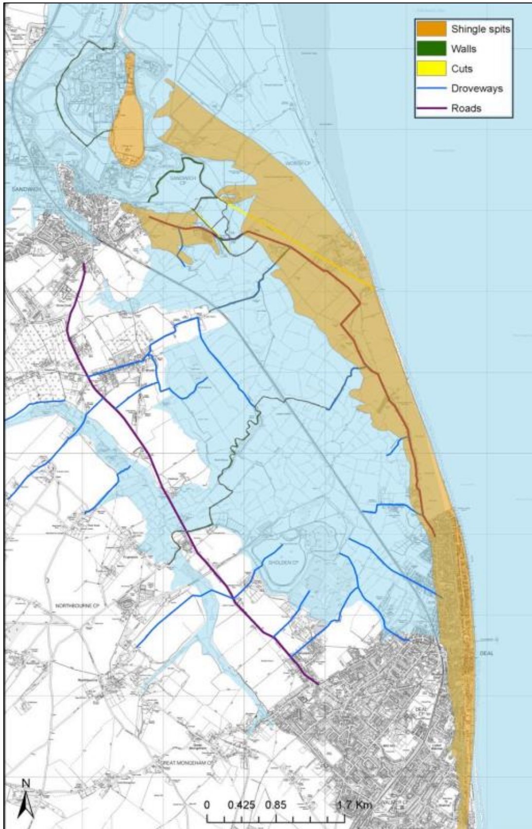
Figure 34 - Lydden Valley and the Mouth of the Wantsum showing Shingle Spits, Historic Sea Walls and Droveys
